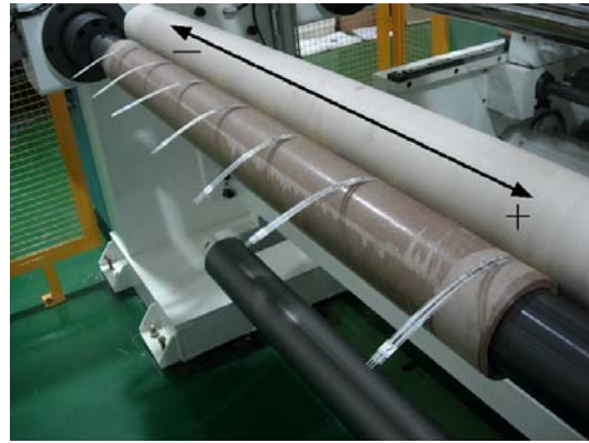
Fig. 24. Measurement of NIT by using FSR.
