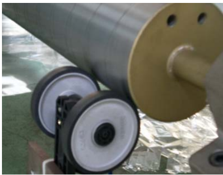
Fig. 20. Encoder for measurement speed of idle roller.
